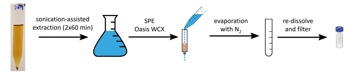
250 mg sediment 2x5 mL 1 M HCl in MeOH + surrogate-mix 10 mL extract + 100 mL buffer (citrate, pH≈5.5) 6 mL extract (2% FA in ACN)
