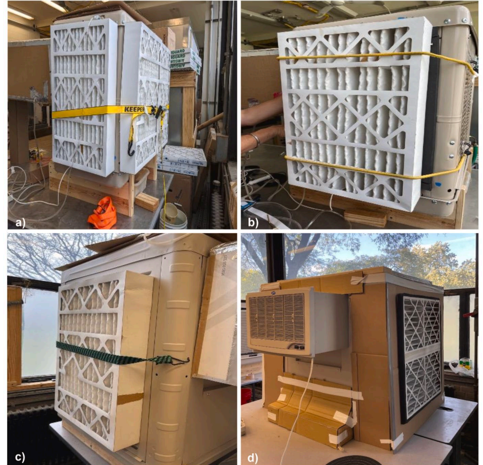
(a) tie-down ratchet straps, (b) bungee cords, (c) bungee straps, and (d) custom plenum-like intake and housing for filters
